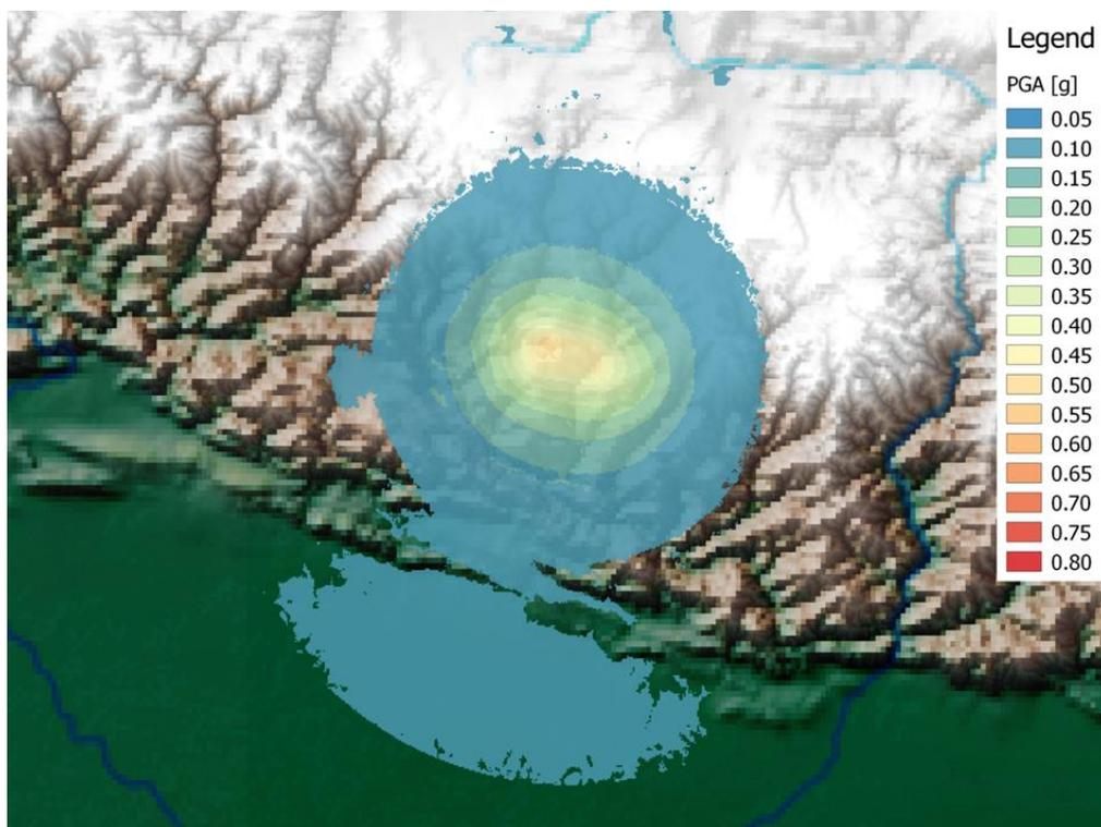
Figure 2: PGA Map (ground motion, g) of the M7.3 earthquake of May 12th, 2015.
