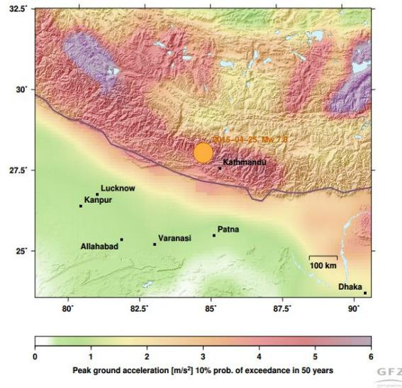
**Figure 15: Peak ground acceleration probability.** For the region of the present event, the global seismic hazard map (GSHAP) shows a probability of 10% for exceeding peak ground accelerations of 5 m/s<sup>2</sup> within 50 years.
