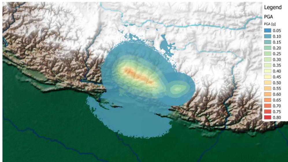
**Figure 19: PGA modelling of the M7.8 earthquake on 25.04.2015 and the M6.7 aftershock**
