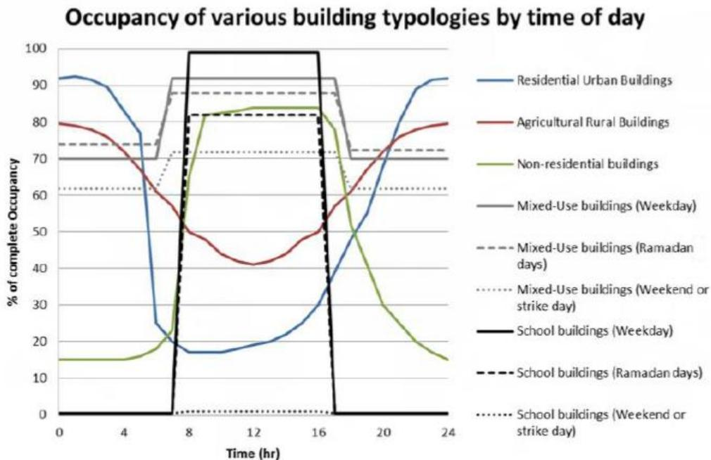
**Figure 8: Occupancy of various building typologies by time of day showing the differences between typologies on weekends and during the week. These combine data from Coburn and Spence (1992) and Ara (2013) in Bangladesh.**
