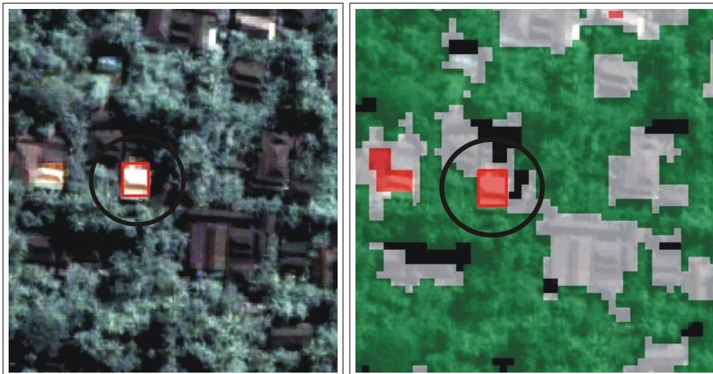
Figure 3. Segmentation and classification applied on multispectral Quickbird satellite images. In the left picture a image object was segmented using a scale parameter of 15 (red square), in the right picture the image object was classified as a red house.
